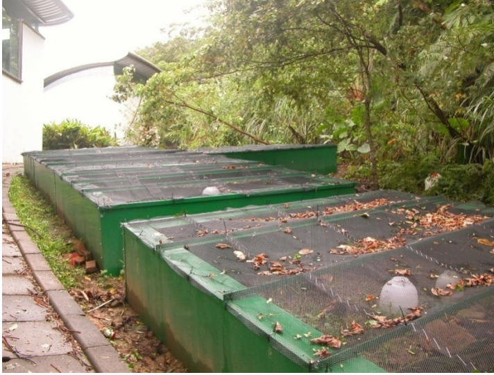
Fig. 1. Outdoor enclosures. The outdoor enclosures were iron-made (width \times length \times height = 3 m \times 3m \times 0.7 m). The button sides of the walls in each enclosure were set underground into 10cm deep, and their upper sides were folded 20 cm inside. The lid made of plastic mesh (pores = 1 cm in diameter) was used to cover the enclosures to prevent predators and human disturbance and to prevent animal's escape from the enclosures.
