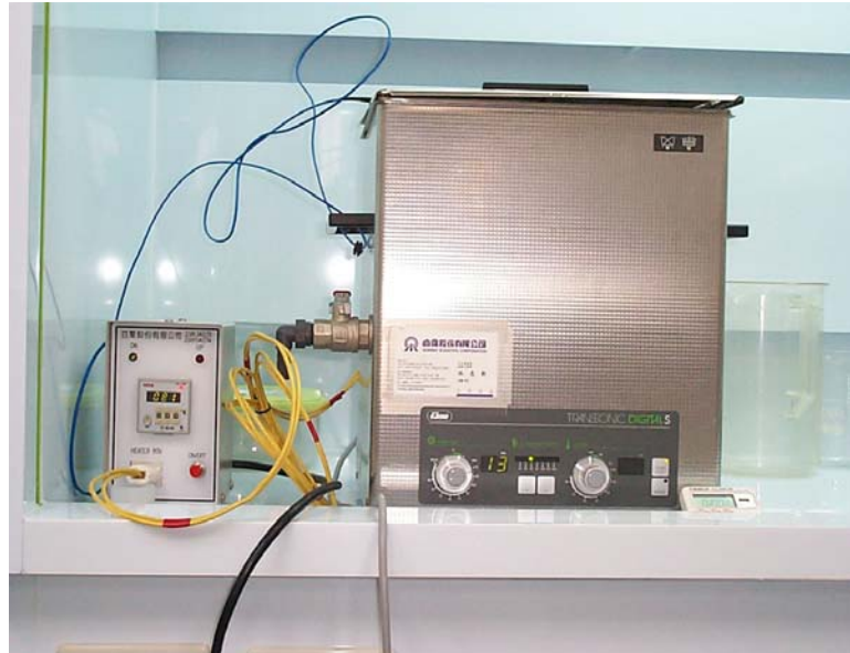
Figure 3-16. Wet etching facilities with ultrasonic agitation.
