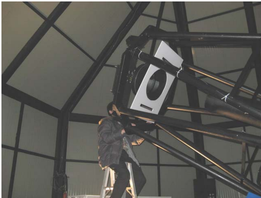
figure 4-3 The front face of double slits mask mount on LOT
