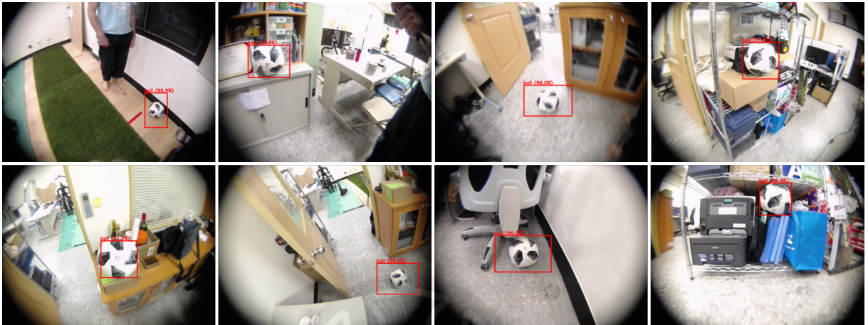
Figure 2.22: The perception system results demonstrate robustness in challenging scenarios, including scenes with similar colored objects, a cluttered shelf, and blurry images
