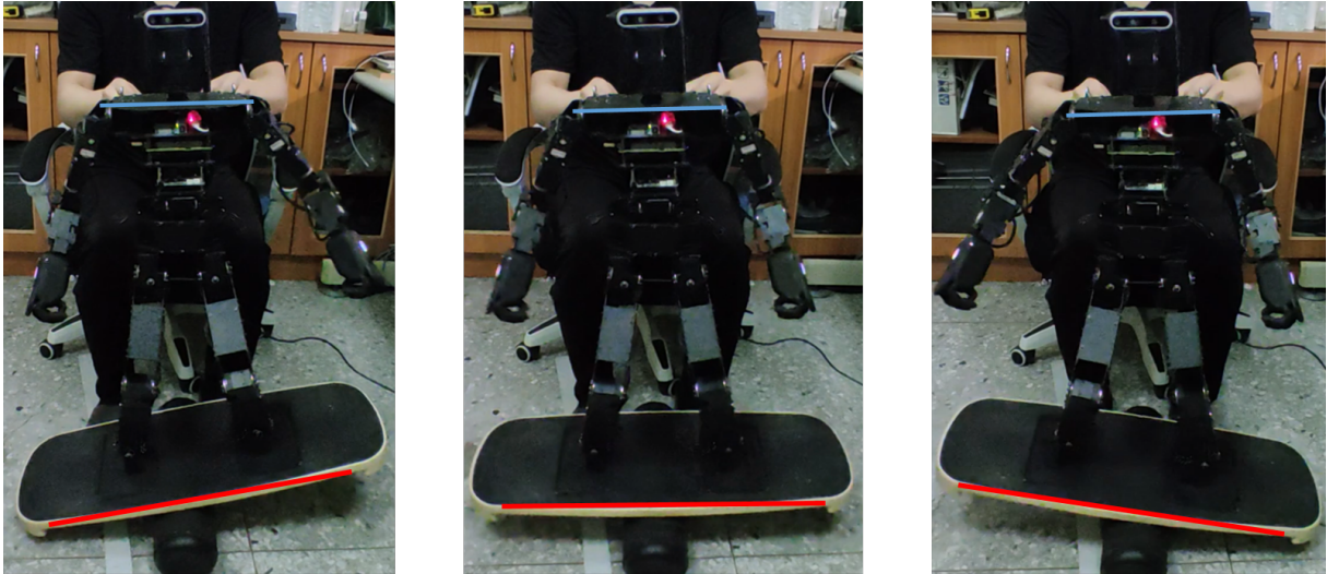
Figure 4.7: The result of the PD controller maintained parallel to the ground for the robot body
