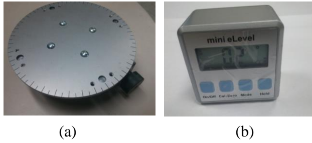
Figure 7.21. Angular measurement tools (a) electric rotary plate (b) electric angle meter.
