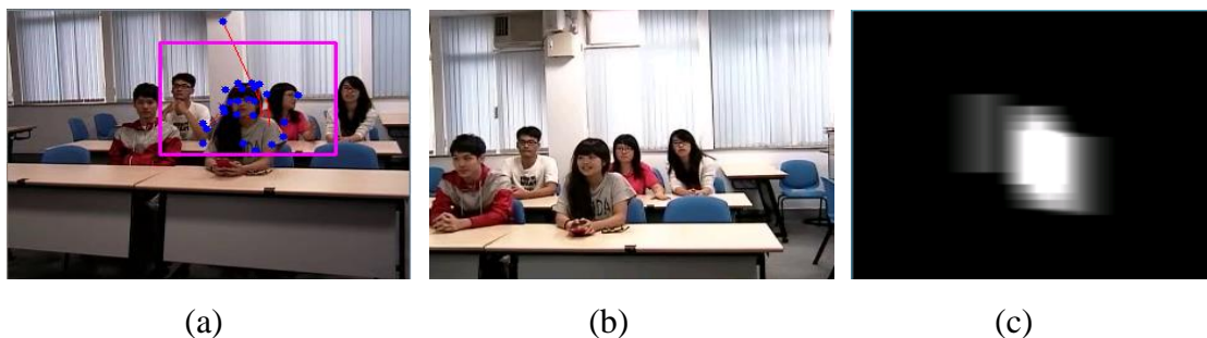
Figure 4.25. ROI selection (a) ROI detection result (b) the shot after camera steering (c) the attention map for selection.
