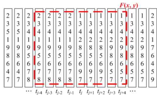
Figure 7. An illustration showing the convolution of the filter F and the target video T . The dashed square indicates the range of F , and t_j is the ordinal signature of the j -th frame in T .
