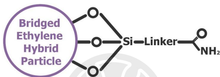
Figure 8. Structure of the Amide-Bonded Stationary Phase.
